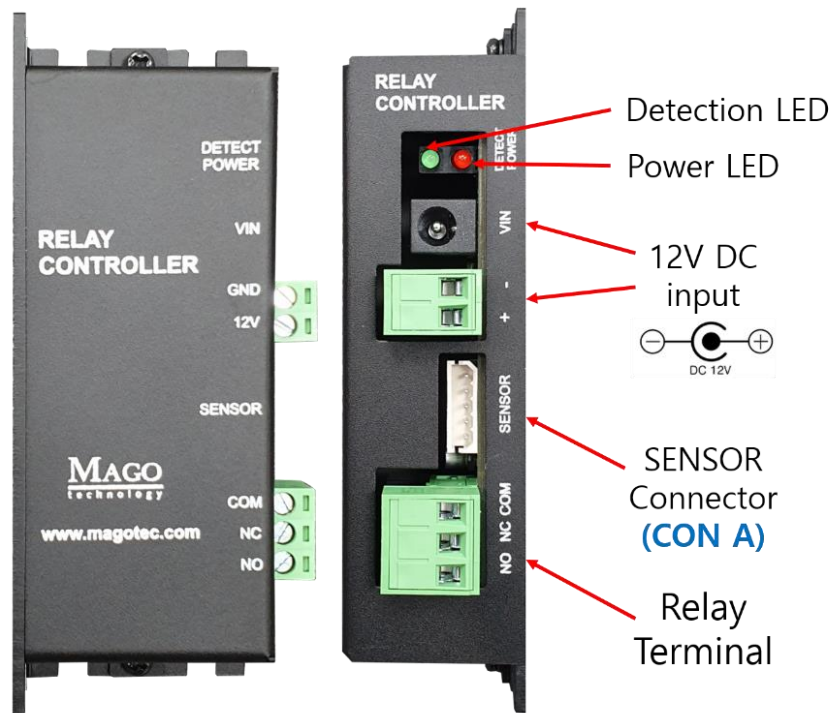
<Fig. 3 CARDET relay controller>
